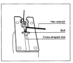
Tilt the base until the desired bevel angle is obtained. The edge of the motor housing indicates the bevel angle by graduations. Then tighten the bolt to secure the base.
